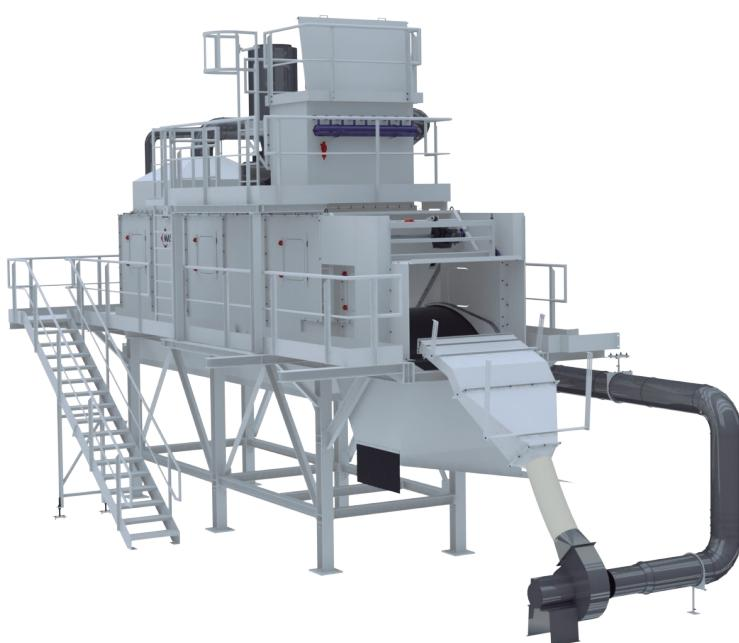
The Windsifter is a rugged equipment with great capacity to separate the light material from the heavy one. The aim of which is the separation of the inert material (stones, scrap, stainless steel) so availability and durability of the secondary shredders of alternative fuels production lines can be increased, thereby assuring a low operating cost.
